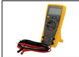
Multimeter/Fluke/179 Capacitance Measurement (Capacitor)
